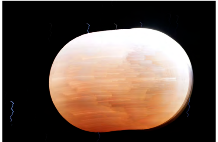
This is a blended composite of a series of 79 photos of the eclipse that John Baker took over a 40 minute period. The interest in this photo is that it demonstrates drift in the mount/drive of the 16" telescope. Note the trail of the stars. If the mount were properly aligned and the drive had been operating smoothly, the star should appear as a point. Slight motion of the Moon would be expected.
